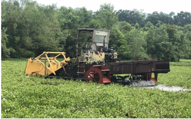
Figure 3. Mechanical removal of water hyacinth at Blackwater Conservation Area (Source: BREC staff)
